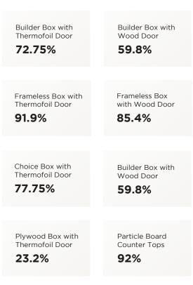
The Framed Builder Cabinet and Frameless Cabinet utilize particle board construction, and when combined with our thermofoil doors manufactured using MDF, provide a high recycled content.
